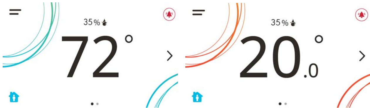
Figure 12: Thermostat controller home screen in cooling mode (left) and heating mode (right)
